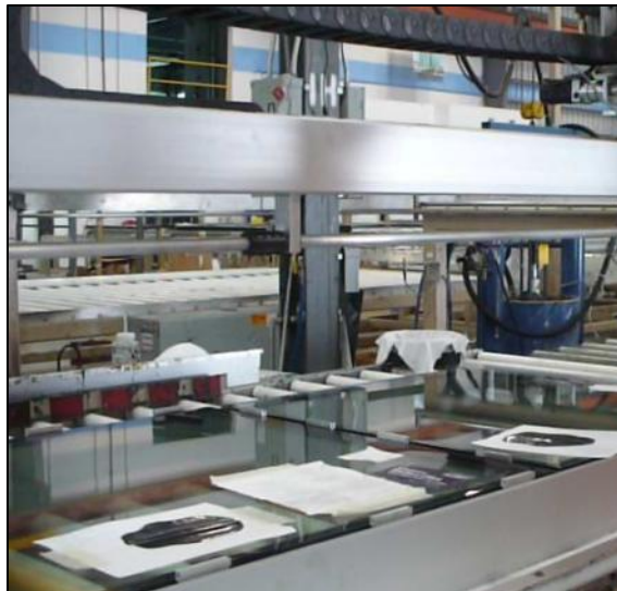
Figure 36 - Sealant Curing on Paper. Courtesy SGH.
